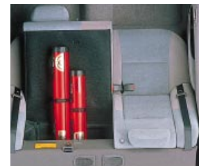
Reclinable rear seat, split at a 6:4 ratio, with a "trunk-through" function
