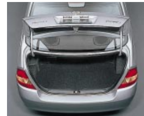
Luggage space with plenty of width and length thanks to the smaller battery
