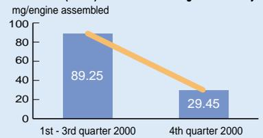
VOC-HAP emissions were reduced when a specialized blend of alcohol lubricant was replaced with common rubbing alcohol for tube installation
