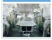
After the body is washed, undercoat, intermediate and topcoat are applied to create a high-quality surface. Waterbased paint has made this process even more environmentally friendly.
